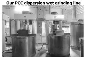
During the wet grinding process, we add several types of chemicals such as dispersing and binding agents into the mixture based on our formulation. These chemicals are added to ensure that the calcium carbonate particles remain dispersed for a certain time in the liquid mixture. Our CC dispersions have a shelf life of 4 months before the particles start to settle down and coagulate.
