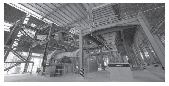
Our GCC production lines are equipped with air classifiers to separate the GCC into different size classes. The air classifier uses an air cyclone and gravitational force within the machine to separate light weight ultrafine particles and heavy coarser particles.
