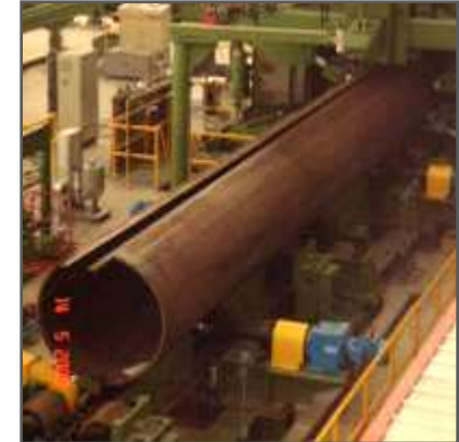
Zhongyou BSS (Qinhuangdao)'s plant started making LSAW pipes
