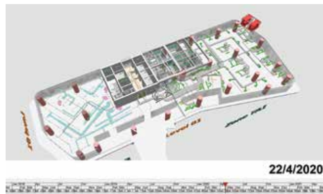
4D BIM simulation of typical floor construction cycle
