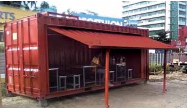
Portable Rest Area Fabricated From Used Shipping Container
