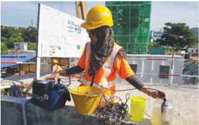
In Situ Total Suspended Solids and Water Turbidity Testing
