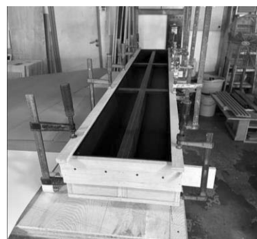
Assembly of wooden components into semi-finished furniture
