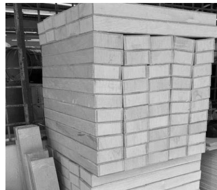
Semi-finished wooden components to be used for further assembly into furniture and fixtures
