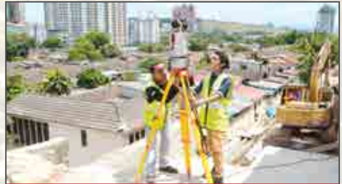
The Terrestrial Laser Scanner (TLS) uses 3D laser technology and provides accurate mapping data
