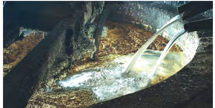
● Blending of molten tin in refinery kettle
