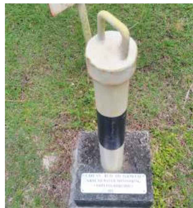
Borehole for groundwater monitoring.
