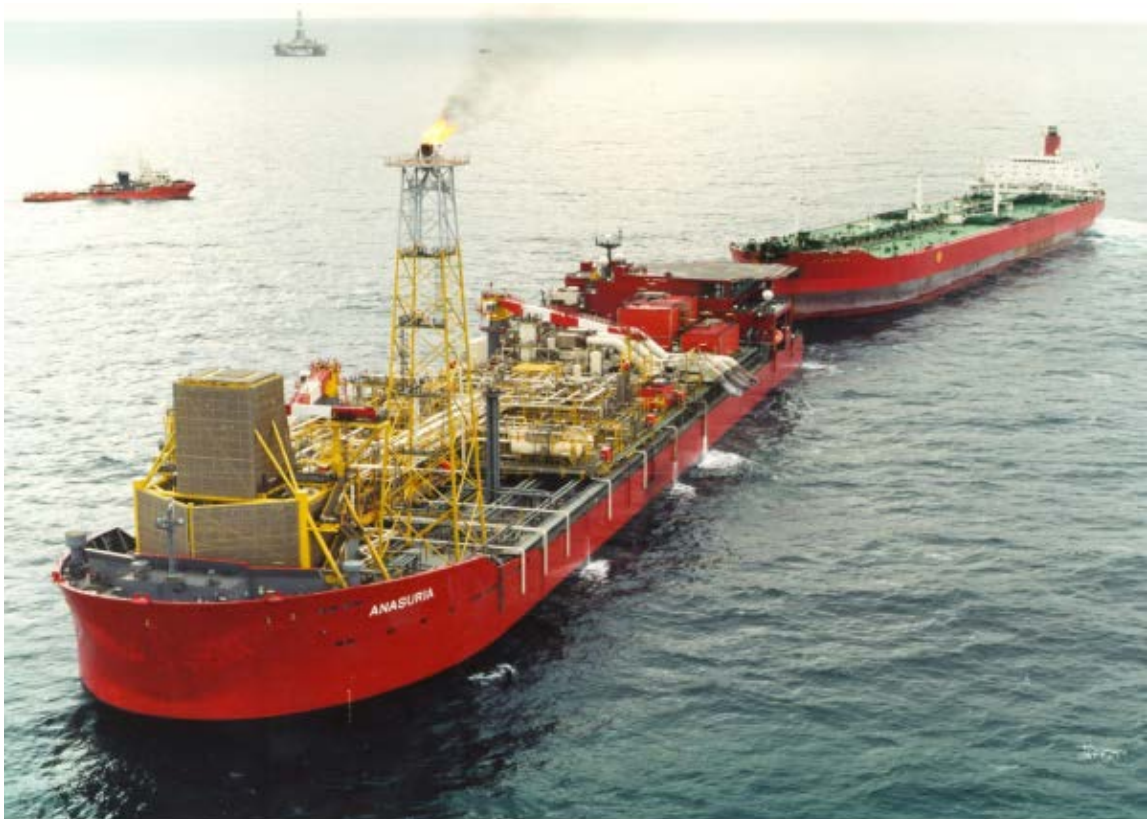
Anasuria FPSO in the Central North Sea during a crude oil offtake
