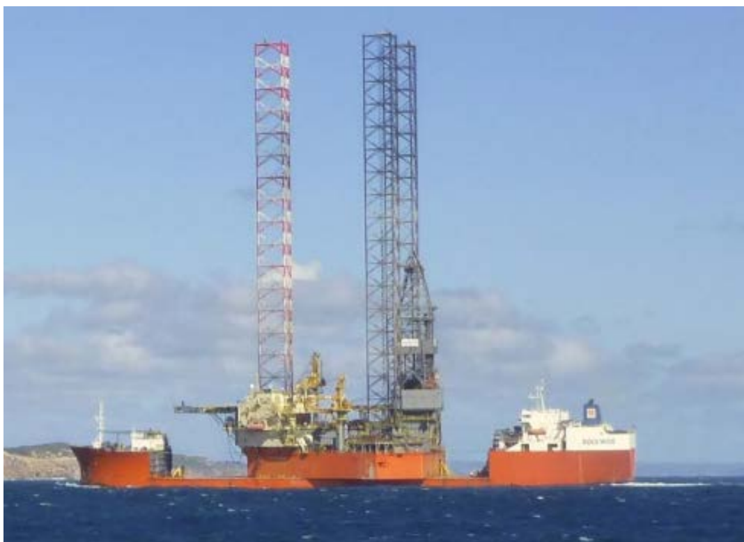
West Telesto being towed on a Heavy Lift Vessel into Port Phillip Bay, Melbourne
