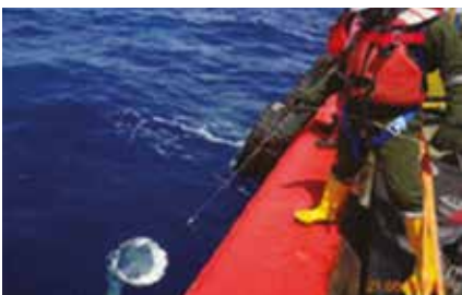
Deploying plankton net through the surface water.
