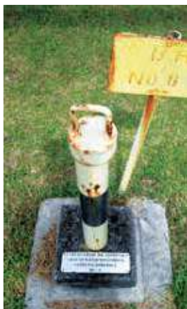
One of the many boreholes in LCOT constructed to monitor our groundwater quality.
