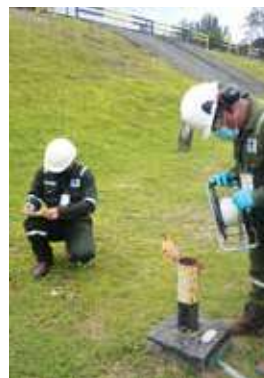
Groundwater monitoring works being carried out in LCOT. Water depth measurements are taken prior to the purging of the groundwater wells. The measurements attained are used to determine the volume required to purge.
