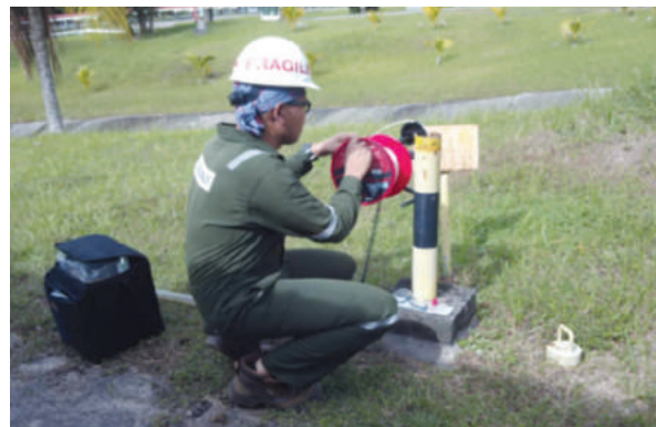
Groundwater Monitoring in progress: Water depth measurements are taken prior to the purging of the groundwater wells. The measurements attained are used to determine the volume of water required to be purged.
