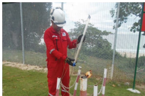
Groundwater Monitoring in progress: Bailers are used to purge and sample groundwater from the respective wells. Samples are contained in sampling bottles with the respective parameter's preservatives.
