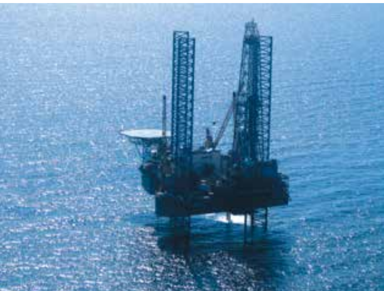
Figure 4: The Aban VII, an independent leg cantilever jack-up drilling rig on location in Block 50 Oman
