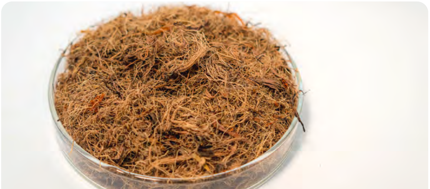
Fibres from palm oil used as fuel for boiler systems.
