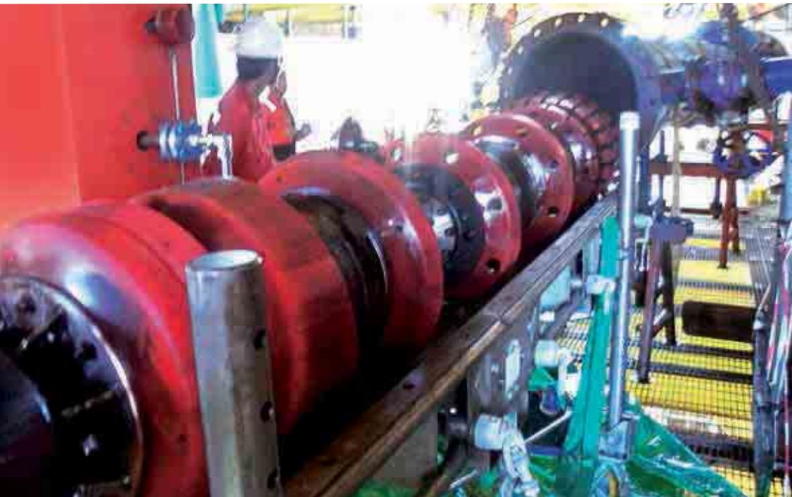
■ Loading of an intelligent pipeline inspection gauges
